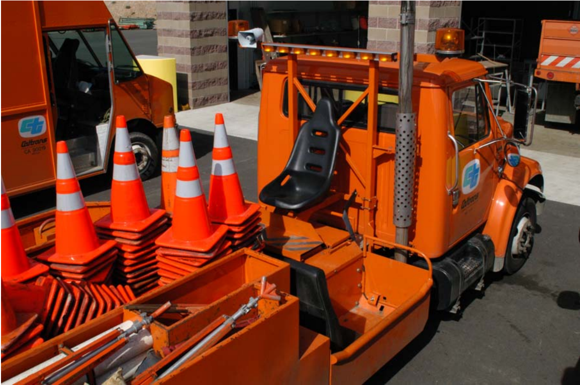
Figure 4-1 Caltrans high capacity manual cone truck (Oakland Bay Bridge)
