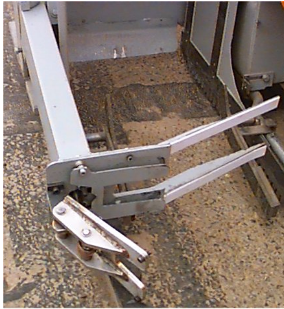
Figure 2-17 Retrieval arm in cone retrieval position
