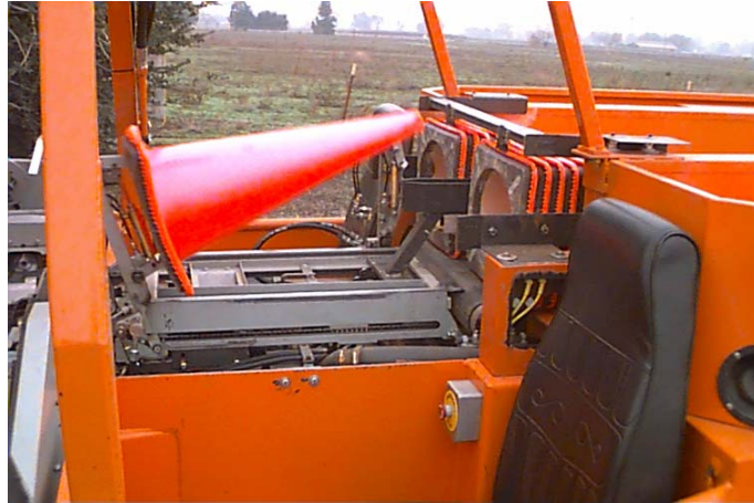
Figure 2-13 Stowage system operating without covers
