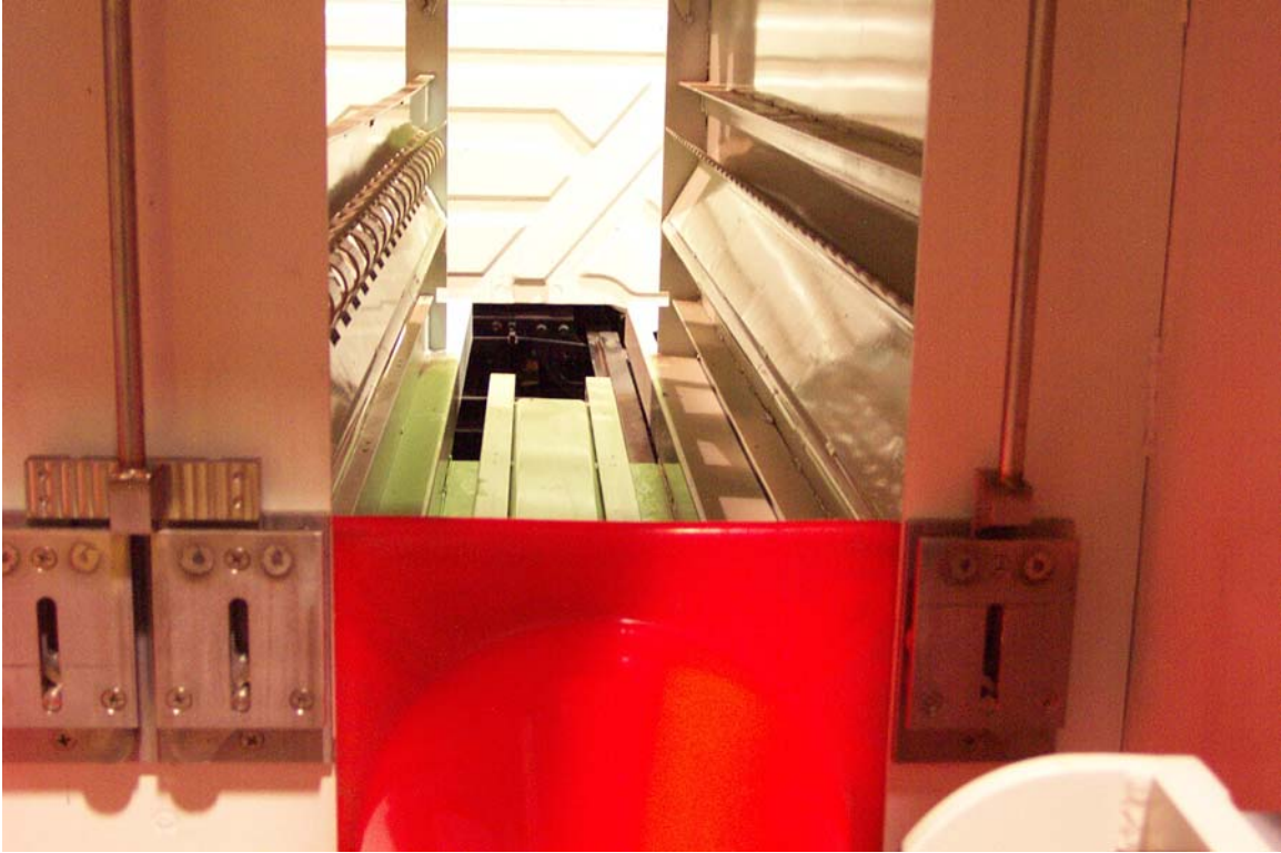
Figure 4-15 View showing hinges (cone shelves) retracted
