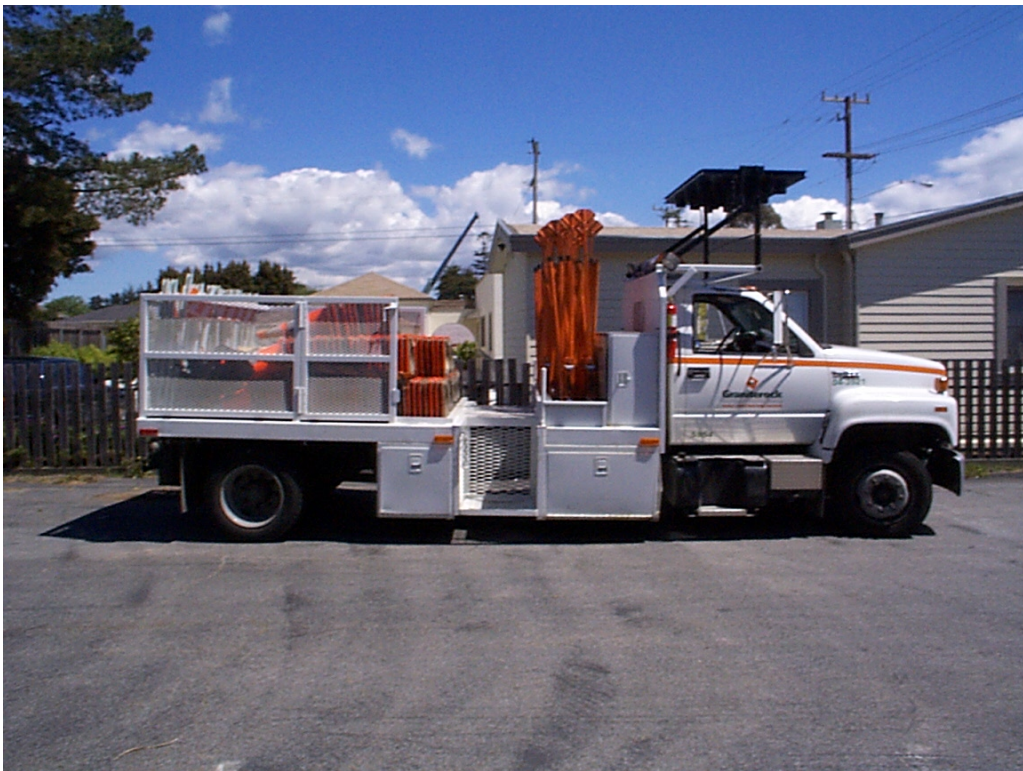
Figure 4-2 Commercial cone truck with 400 cone capacity
