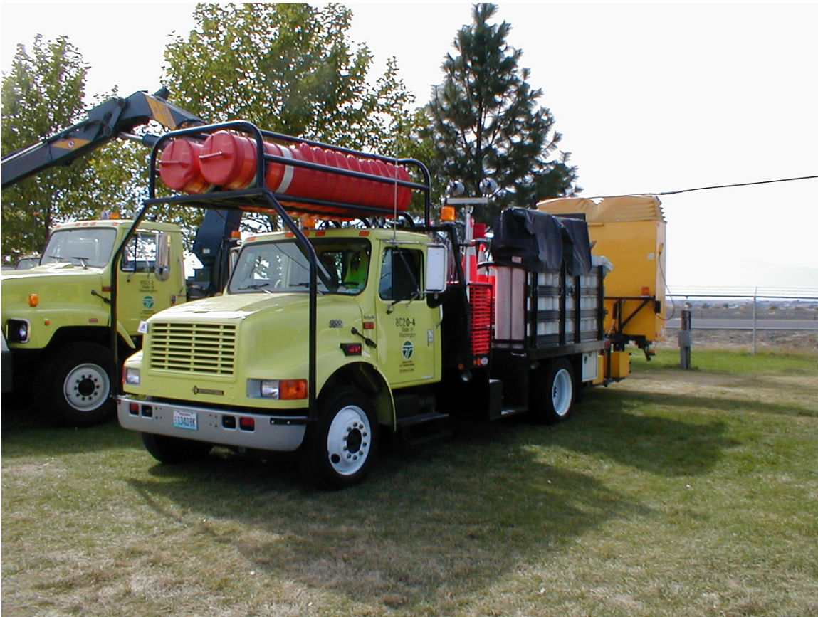
Figure 4-3 High capacity cone truck used by Washington DOT
