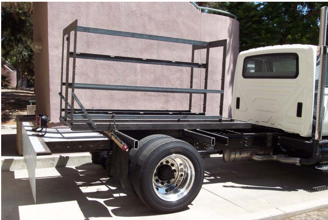
Figure 4-12 Storage framework before attachment of panels
