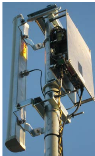
Figure 4.4 AHMCT 5.8 GHz point-to-point communication experimental setup
