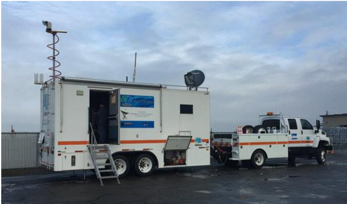
Figure B.1: A Caltrans SATCOM trailer
