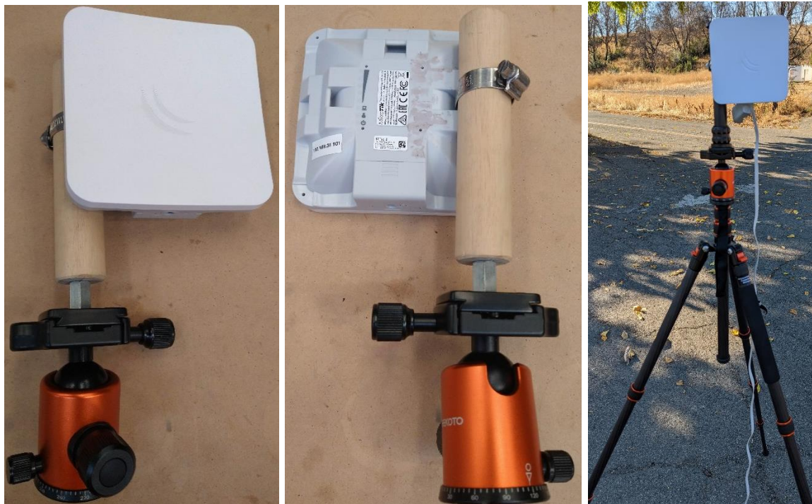
Figure 2.7: MikroTik SXTsq 5 High Power with integrated 5 GHz 16 dBi antenna mounted on a tripod
