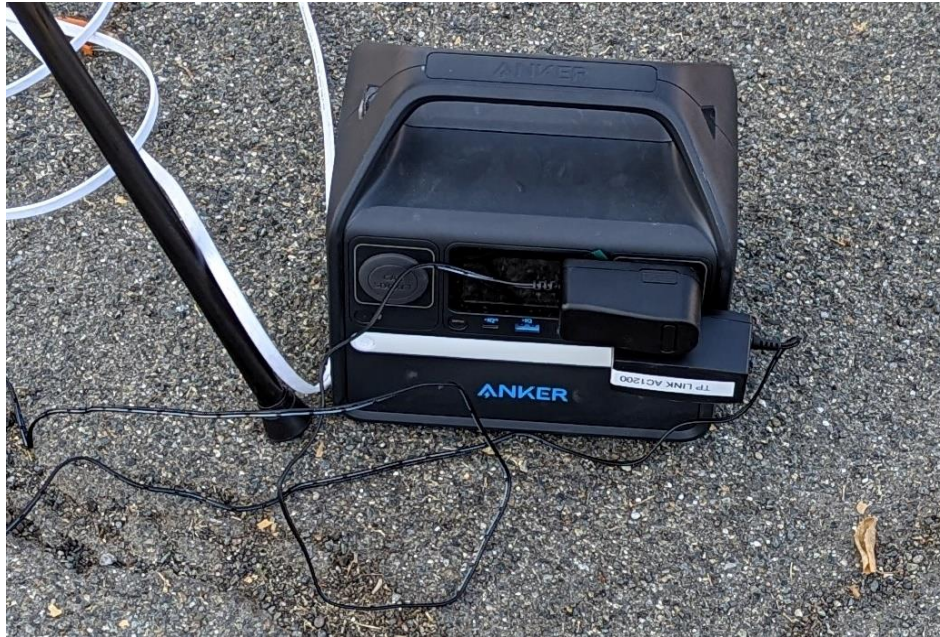
Figure 2.10: COTS battery power station (Anker 521) used to power the Wi-Fi Bridge and Wi-Fi Repeater
