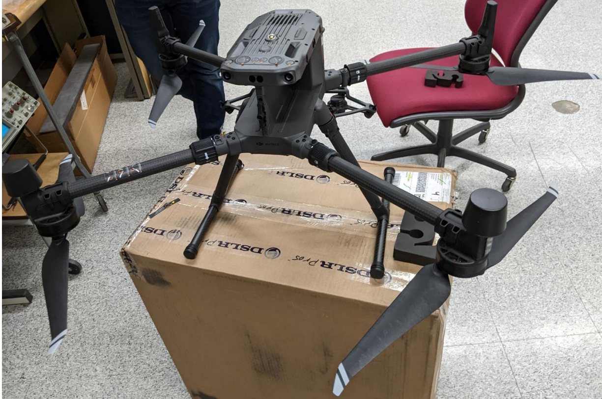
Figure 4.3: DJI Matrice 300 RTK with legs attached and motor arms and props extended. Here, battery bays are empty.
