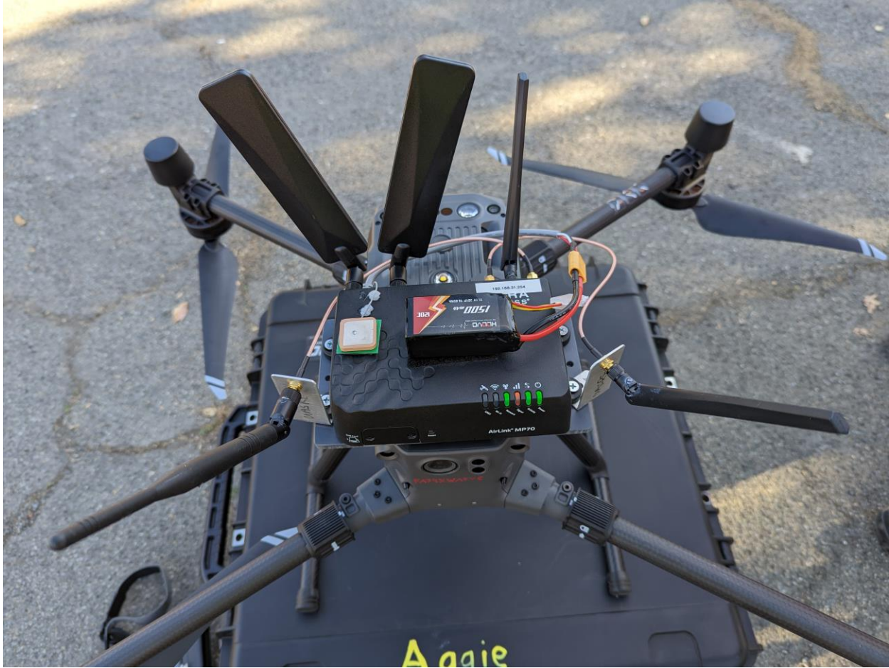
Figure 2.2: Sierra Wireless MP70, Wi-Fi antennas, and battery secured to DJI Matrice 300 mounting plate
