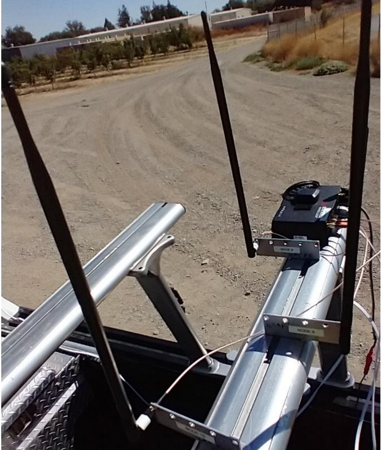
Figure 2.1: Experimental setup to investigate Wi-Fi range with different Wi-Fi antenna and antenna spacing. Sierra Wireless MP70 with LTE, Global Navigation Satellite Systems (GNSS), and 9 dB gain Wi-Fi antennas with 9-inch spacing.
