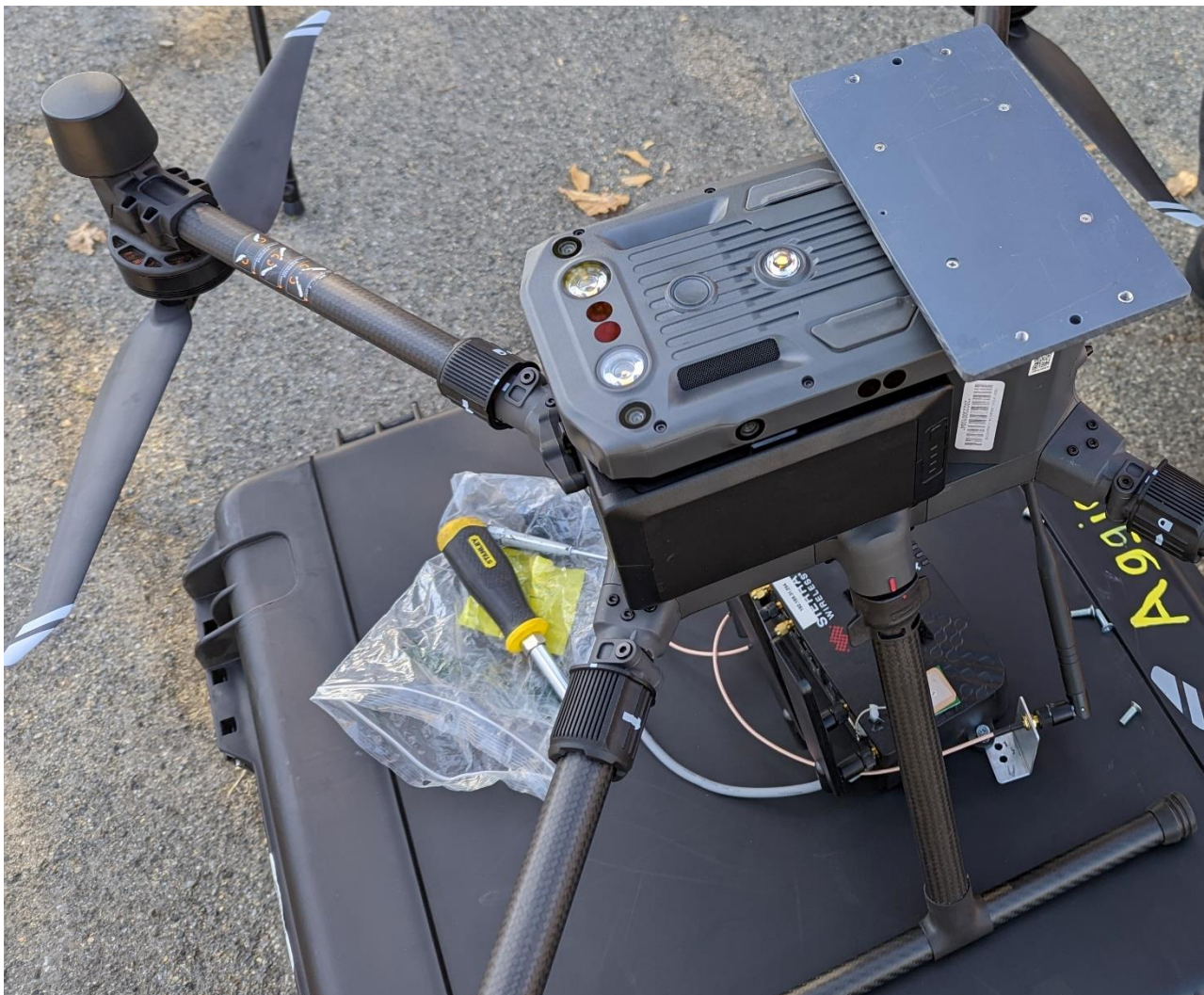
Figure 2.1: UAS repeater to DJI Matrice 300 mounting plate secured with four M3x0.5 mm screws
