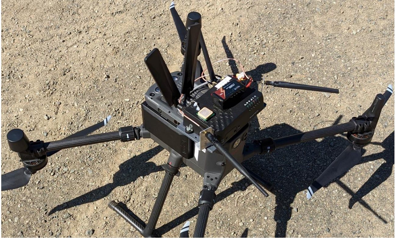
Figure 2.5: Sierra Wireless MP70 with LTE, GNSS, and 5 dB gain Wi-Fi antennas mounted on the UAS. The LTE antennas were changed to the final version - compare to the LTE antennas shown in Figure 2.4.
