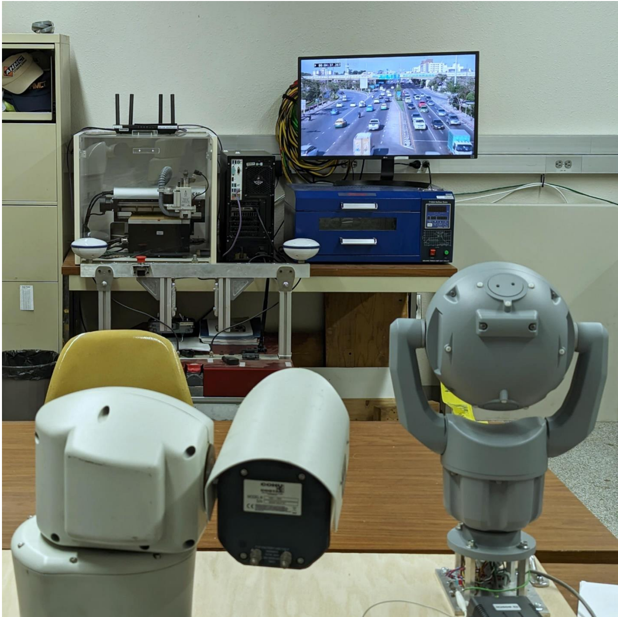
Figure 3.3: CCTV devices aimed at the test display
